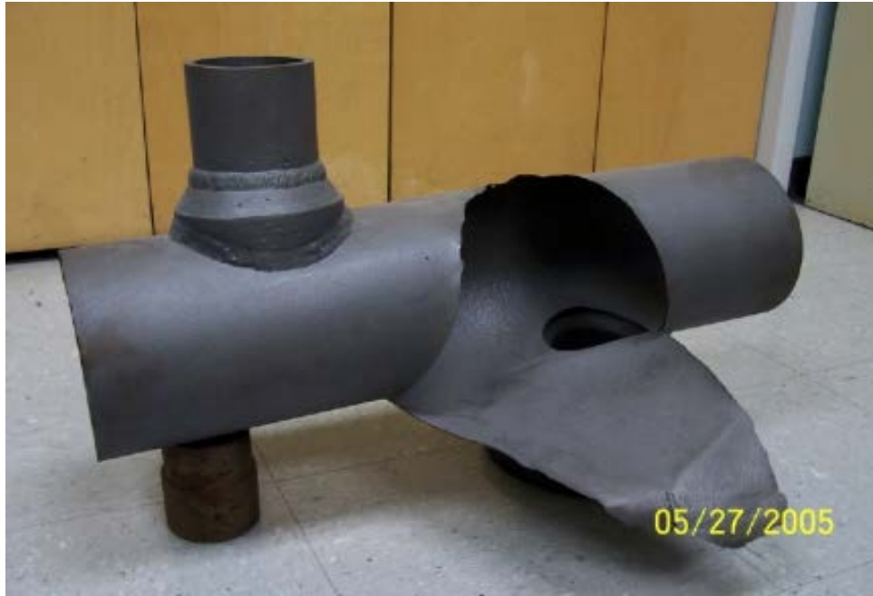
Figure 1—NPS 8 Carbon Steel Piping Failed Due to Sulfidation Corrosion (H 2 Free)
