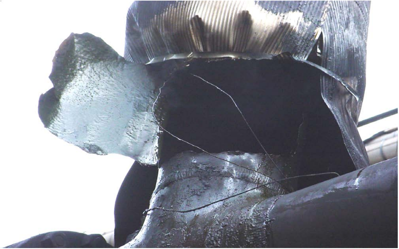
Figure 3—FCC Fractionator Bottoms Carbon Steel Piping Operating at 150 psig (1 MPa) and 650 °F to 700 °F (340 °C to 370 °C)
